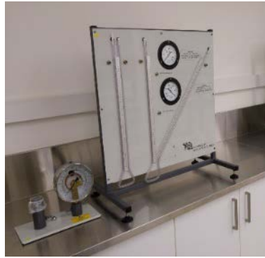
Figure 2: Pressure Measurement apparatus (right) and Calibration of a Pressure Gauge apparatus (left). The pressure measurement apparatus was purchased from TecQuipment Ltd.
