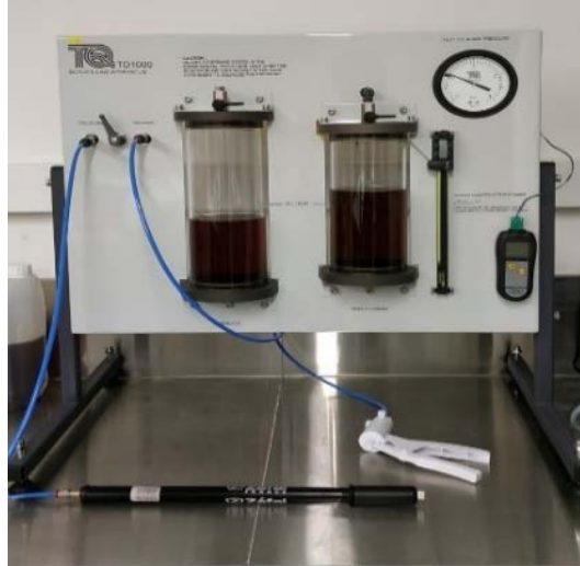
Figure 7: Experimental equipment for the verification of Boyle's.
