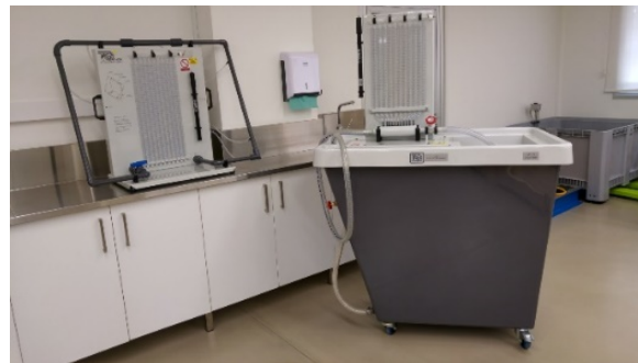
Figure 1: Pipework Energy Losses apparatus (left) and Venturi Meter fits on Hydraulic Bench (right). Both experimental apparatus were purchased from TecQuipment Ltd Company.
