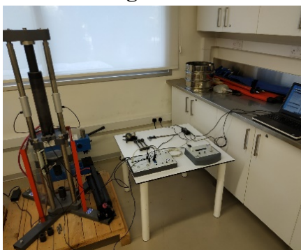
Figure 3: The experimental set up of the Tensile Testing purchased from TecQuipment Ltd Company (left) and an experimental stress-strain curve acquired from a tensile testing on a steel material (right).
